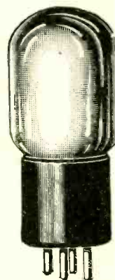
High-mu tube for battery operation, equivalent to the 240, but listed as 201A high mu.
